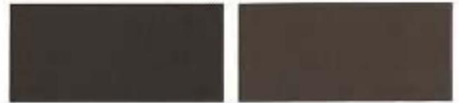
Weathering steel is restricted in applications, because run-off of rusty water from steel surfaces in the initial application period many pollute the surroundings. The WEATHERCOAT method prevents steel from canting such defective run-off. This efficient surface treatment forms a stable rust layer for keeping the beautiful appearance for many
